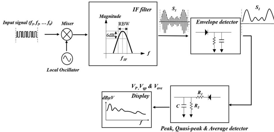
Fig. 11. Operating principle of a spectrum analyzer.
