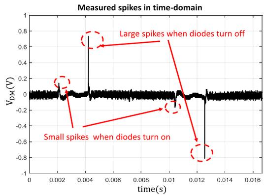
Fig. 6. Measured DM voltage  $V_{DM}$  at the output of a DM noise separator.
