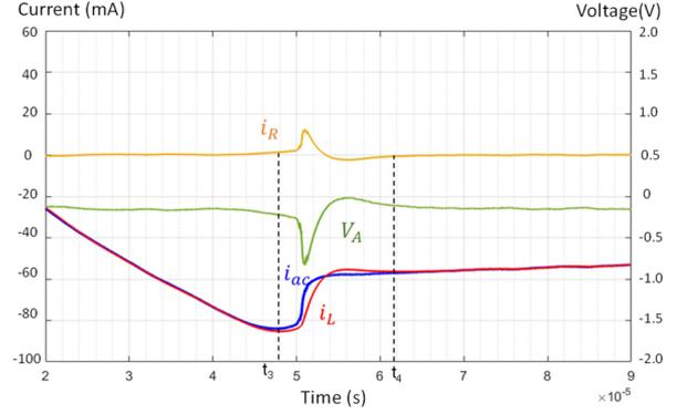
Fig. 9. Simulated currents and  $V_A$  during the reverse recovery transient.
