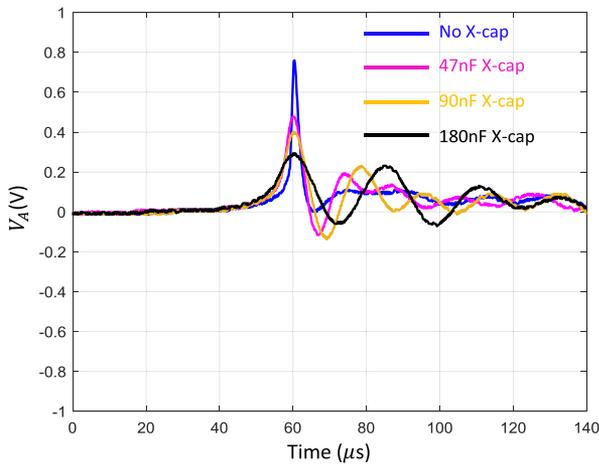
Fig. 17. Measured output voltage  $V_A$  on one LISN with different  $C_X$ .
