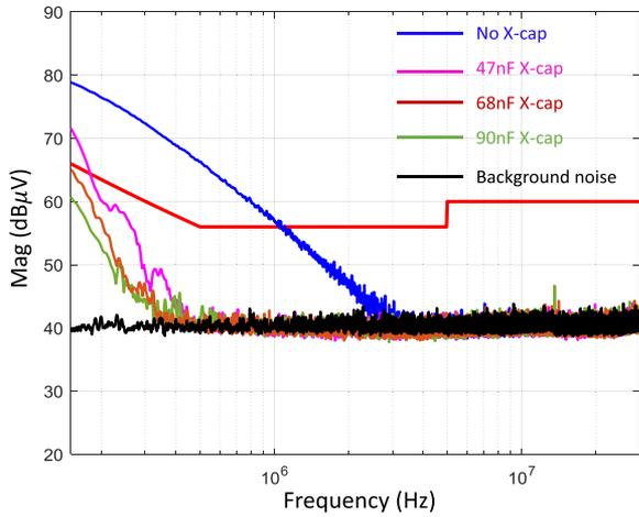
Fig. 16. Measured peak EMI with and without  $C_X$ .
