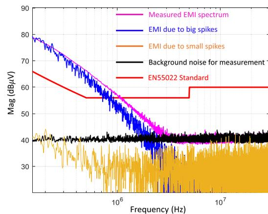
Fig. 7. Comparison of the peak EMI due to two voltage spikes.
