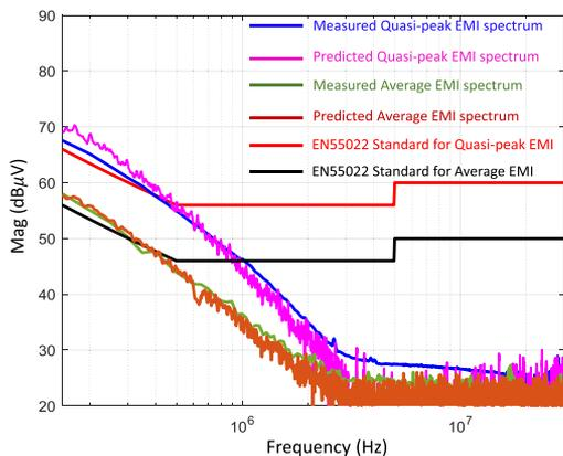
Fig. 13. Comparison of the measured and the predicted quasi peak and average EMI.
