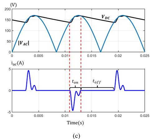
Fig. 1. (a) Flyback converter under investigation with LISNs. (b) Setup for measurement. (c) Voltage and current waveforms of the diode bridge rectifier.
