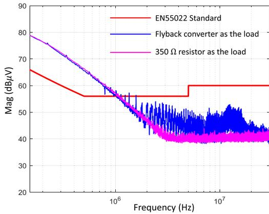
Fig. 5. Comparison of the measured EMI spectra with a resistor load and a flyback converter load.
