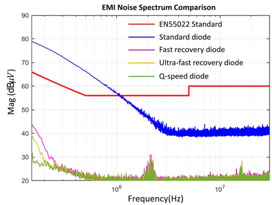
Fig. 19. Comparison of the measured EMI spectra with different types of diodes.
