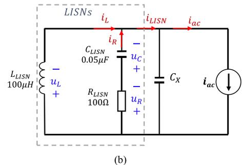
Fig. 14. (a)  $X$ -capacitor  $C_X$  is added between the LISNs and the diode rectifier, (b) DM noise circuit model with an  $X$ -capacitor  $C_X$  applied.
