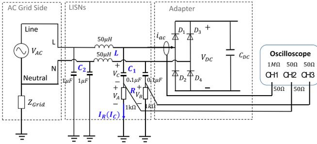
Fig. 3. Measurement setup for  $i_{ac}$  and output voltages  $V_A$  and  $V_B$  of LISNs.
