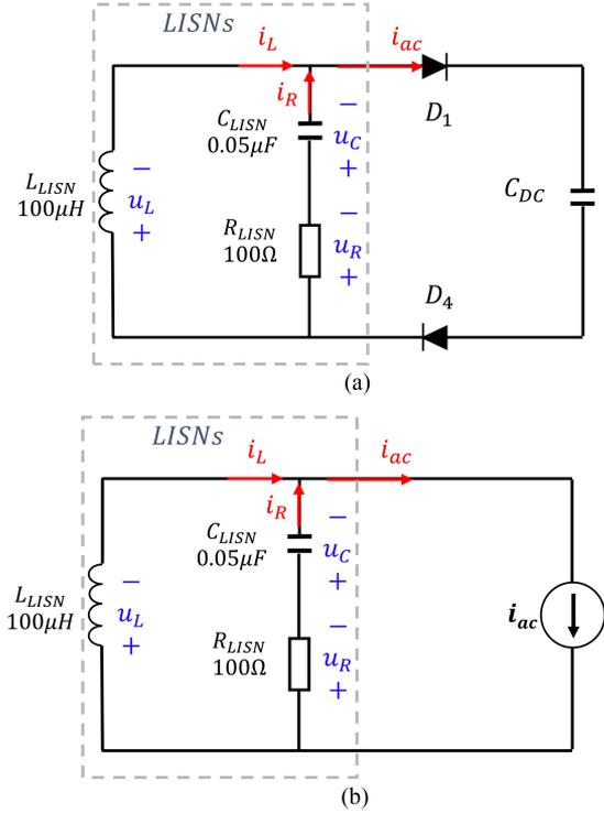
Fig. 8. (a) Circuit model to analyze the impact of the diode reverse recovery currents on the measured EMI. (b) Replacing diodes and  $C_{DC}$  with a current source  $i_{ac}$ .
