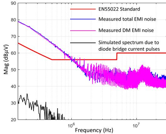
Fig. 2. Comparison of the measured and simulated EMI spectra.
