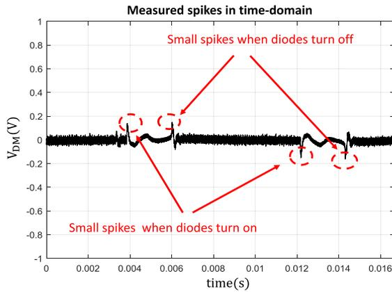
Fig. 20. Measured output voltage of the DM separator with fast diodes.
