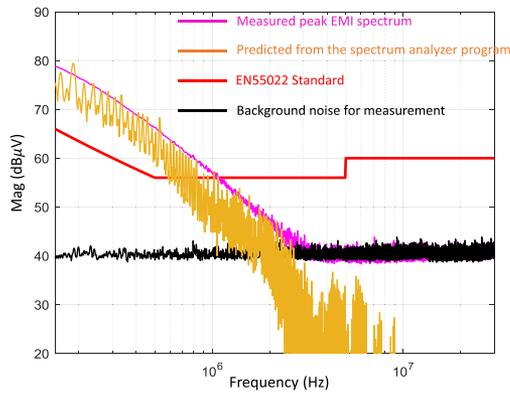
Fig. 12. Comparison of the measured and the predicted peak EMI due to the reverse recovery current of the diode bridge.
