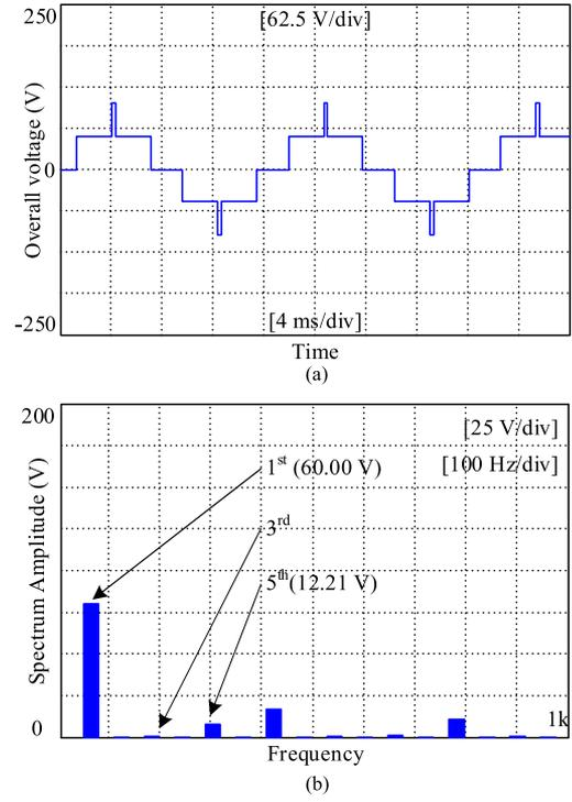
Fig. 20. Simulated steady-state results using the proposed technique in a three-cell CMI to eliminate third harmonic when  $m = 0.94$ , (a) overall voltage waveform and (b) FFT result of the voltage waveform.
