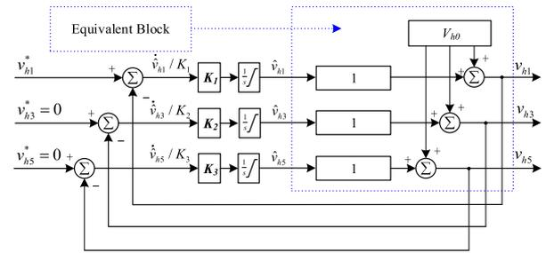
Fig. 10. Equivalent circuit with the decoupling controller.
