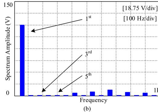
Fig. 12. Simulated steady-state results with fundamental reference as  $v_{h1}^* = 110.7$  V,  $v_{h3}^* = 0$  V,  $v_{h5}^* = 0$  V, (a) overall voltage waveform and (b) FFT results of the voltage waveform.
