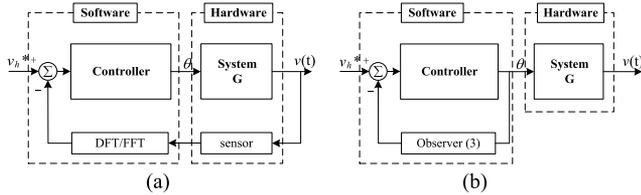
Fig. 4. Control diagram: (a) with DFT/FFT and (b) with an inner observer.
