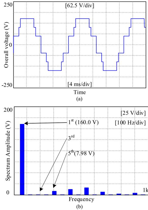
Fig. 19. Simulated steady-state results using the proposed technique in a three-cell CMI to eliminate third harmonic when  $m = 2.51$ , (a) overall voltage waveform and (b) FFT result of the voltage waveform.
