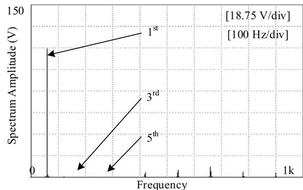
Fig. 13. Measured steady-state results with fundamental reference as  $v_{h1}^* = 110.7$  V,  $v_{h3}^* = 0$  V,  $v_{h5}^* = 0$  V, (a) overall voltage waveform and (b) FFT results of the voltage waveform.
