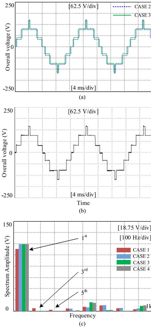
Fig. 22. Simulated and measured steady-state results using the proposed technique in a three-cell CMI with unbalanced dc bus voltages. (a) Overall voltage waveforms with different dc bus voltage conditions, (b) Case 4: a measured output voltage waveform with unbalanced DC bus voltages, voltage feedback and the proposed control loop and (c) FFT results of the voltage waveforms.
