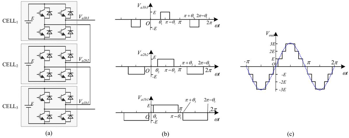
Fig. 1. Topology and waveforms of a three-cell CMI. (a) Topology of a seven-level CMI. (b) Output voltage of one cell. (c) Overall output voltage waveform.
