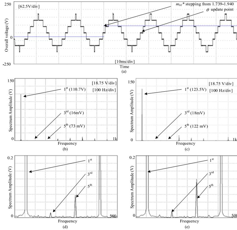
Fig. 14. Dynamic response of the system with  $m_{h1}$  stepping from 1.749 ~ 1.940, (a) overall voltage waveform, (b) voltage spectrum with  $m_{h1}^* = 1.739$ , (c) voltage spectrum with  $m_{h1}^* = 1.940$ , (d) enlarged voltage spectrum with  $m_{h1}^* = 1.739$ , (e) enlarged voltage spectrum with  $m_{h1}^* = 1.940$ .
